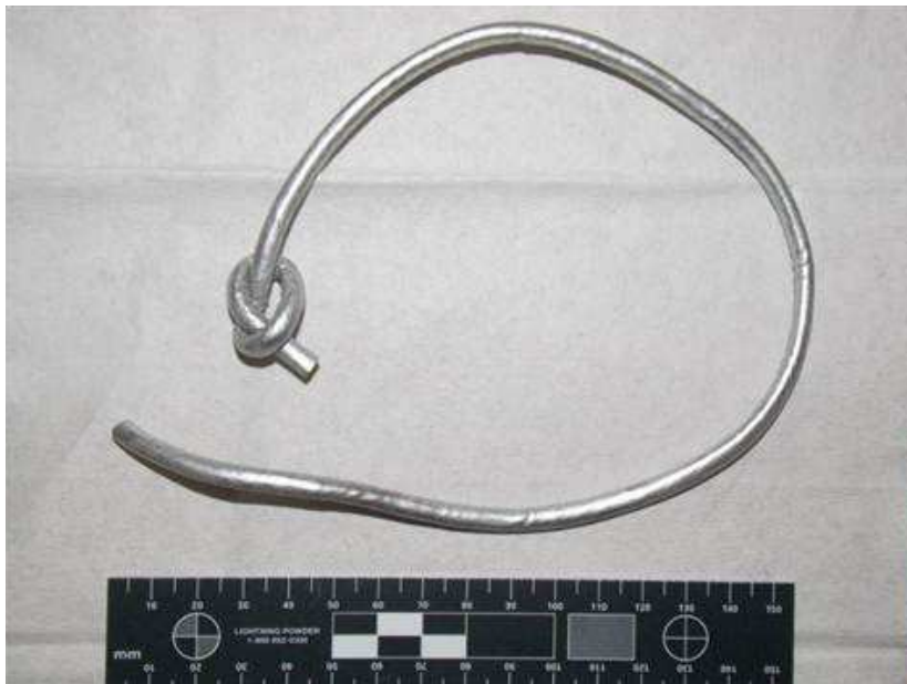
Red detonator cord recovered from the 20 October 2013 incident at Hoodon (below). The det cord is red but covered in TNT/aluminum residue from the main charge.
