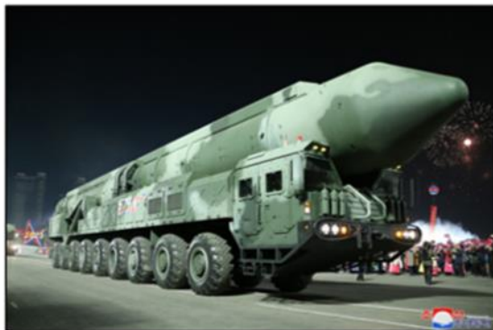
New ICBM in canister on 9-axle wheeled TEL (5 units) This TEL is a slightly different from the Hwasong-15 9-axle TEL
